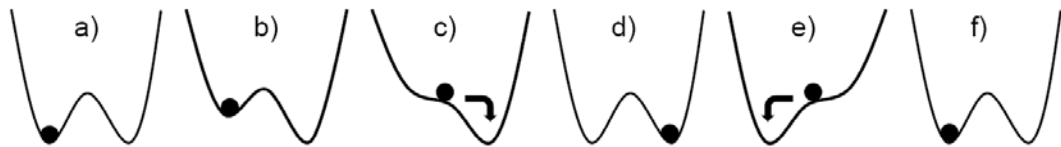
Figure 4. Energy profiles of a bistable system. After saturation the single domain grains of sintered NdFeB magnets can be considered as bistable systems.
