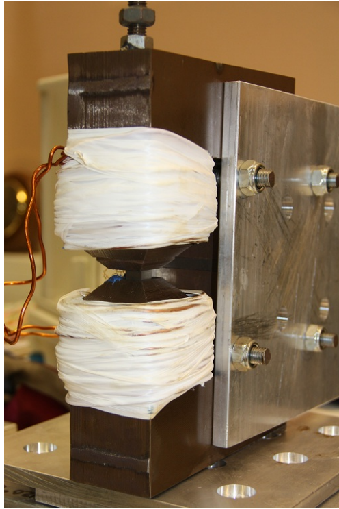
Figure 17. The iron yoke for testing materials in homogenous magnetic field conditions.
