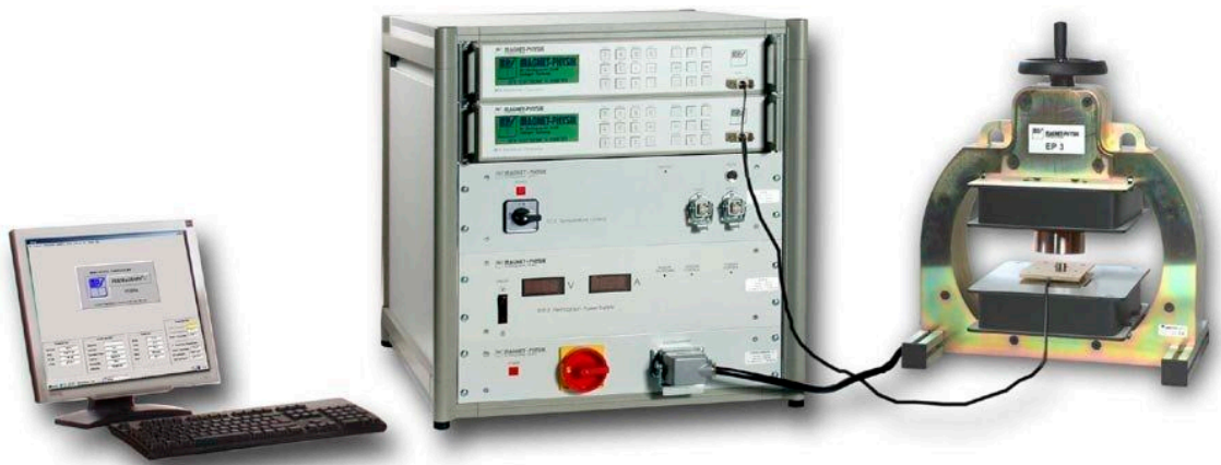
Figure 15. Permagraph C 300 from Magnet Physik used in the BH curve measurements.
